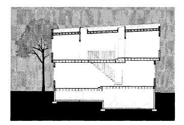
Criteria Addressed: Expanding Upward, Ceiling Height Variety, Opening in Roof, Borrowed Space The floor area of narrow lots is too small to be broken up into celllike rooms containing only one function. Walls chop up the flow of spaces and block off valuable light. However certain rooms must have walls to maintain privacy.
